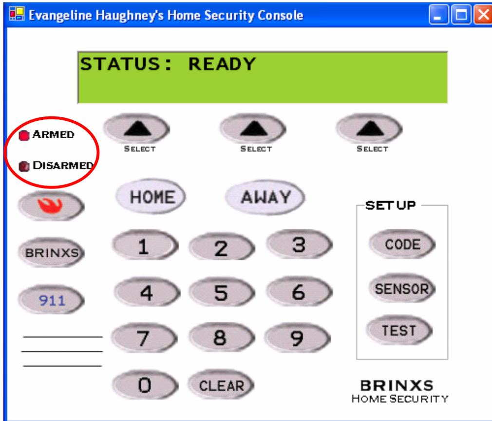
When the user sets the alarm or turns off the alarm, the display indicator lights on the left side of the panel light up.
