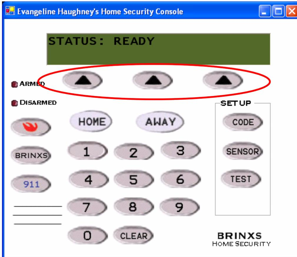
There is a row of three selector buttons immediately below the LED screen. The first row of the LED always contains a status text display. The second row of the LED sometimes contains system responses and options for selection.
